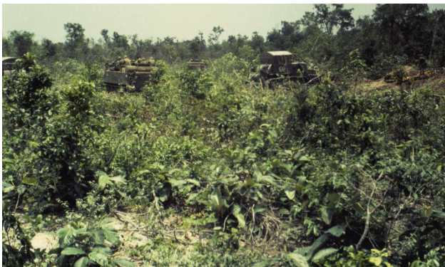
Roam Plows in the Jungle start-1.jpg | Working with the plows was interesting. They would create a temporary base for all of us in the form of a very high berm. Then they would plow down jungle all day, and retreat to the berm line at night. All night you would hear mechanics grinding the plow blades to sharpen them. I believe the plowing was done after it was determined that agent orange was "not a good substance" to use, but i have no proof. (1403x832)
