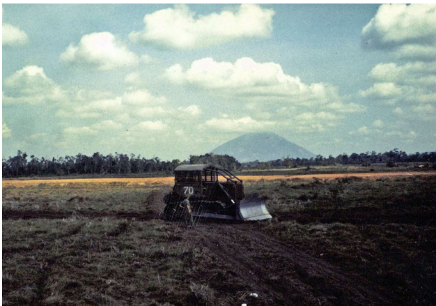
Roam Plows in the Jungle all done w nui ba dinh-1.jpg | Typically the plows would clear a wide zone around roads to prevent ambushes. This once was lush jungle and deny cover to enemy troop movements. (1429x997)
