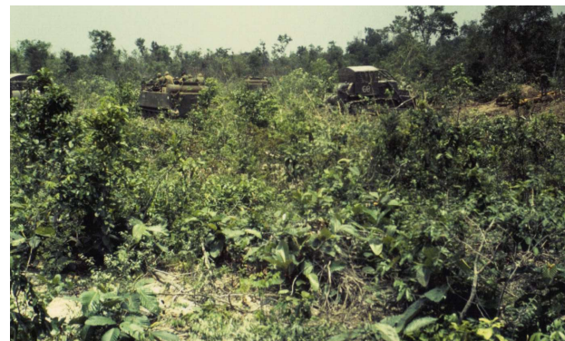
Roam Plows in the Jungle start.jpg | Working with the plows was interesting. They would create a temporary base for all of us in the form of a very high berm. Then they would plow down jungle all day, and retreat to the berm line at night. All night you would hear mechanics grinding the plow blades to sharpen them. I believe the plowing was done after it was determined that agent orange was "not a good substance" to use, but i have no proof. (1403x832)
